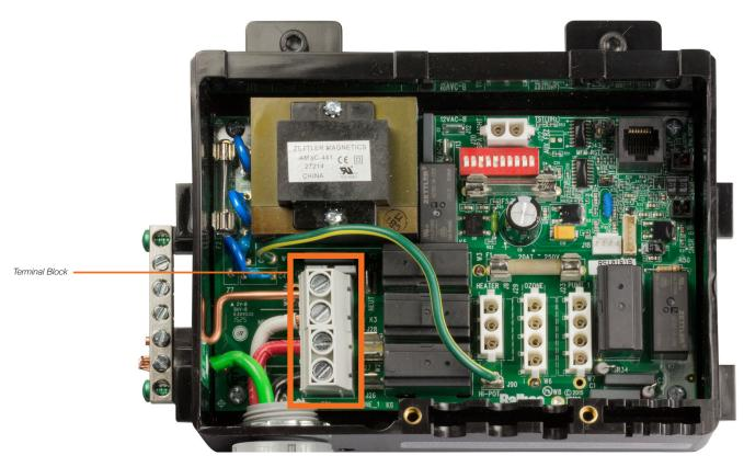
Voltage measurements that vary plus or minus 10% are accurate. For example, if a 240V component is measured between 216V - 264V, the reading is accurate.
