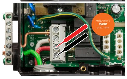
Verify fuse F2 is good by measuring voltage between the terminal block and the fuse. Set the volt meter to AC voltage. Measure voltage on both sides of the fuse. Fuse F2 protects the pump and ozone generator.
